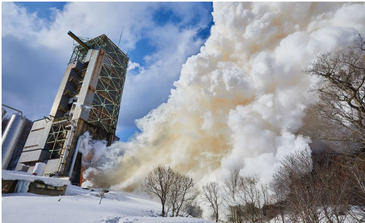
First-stage battleship tank firing test at MHI's Tashiro Test Facility.
