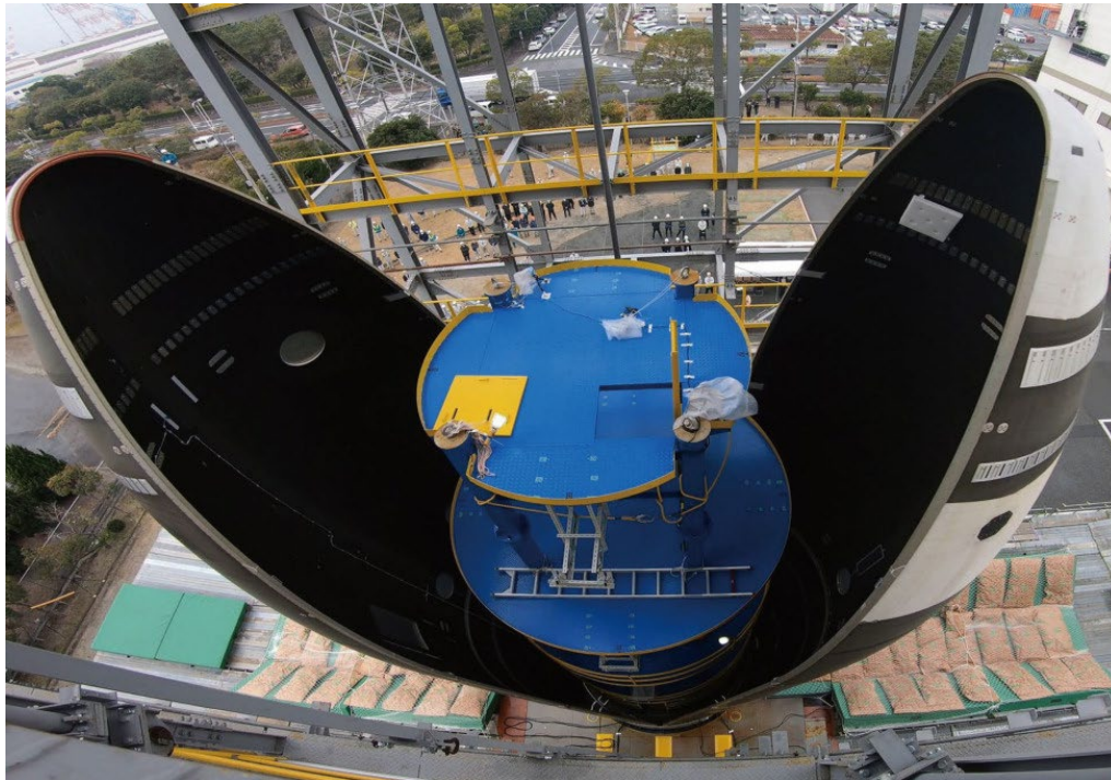
H3 payload fairing separation and jettison test, 17 December 2019.
