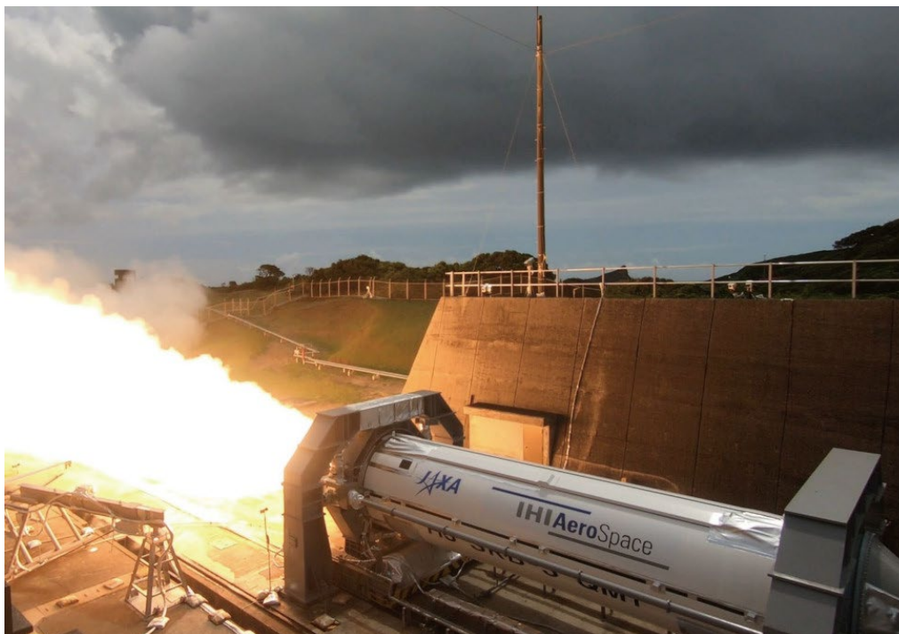
Static firing of the H3 SRB-3 qualification motor, identified in this photograph's source caption as 21 August 2019.
