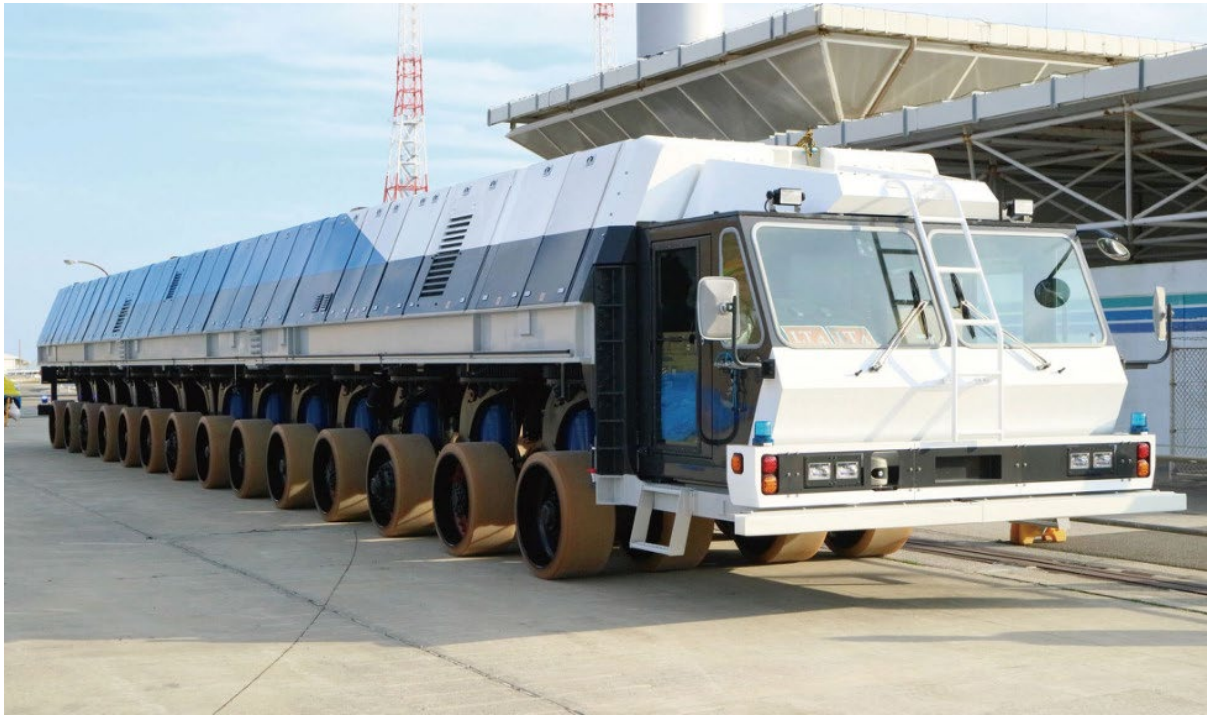
New H3 movable-launcher transporters.
