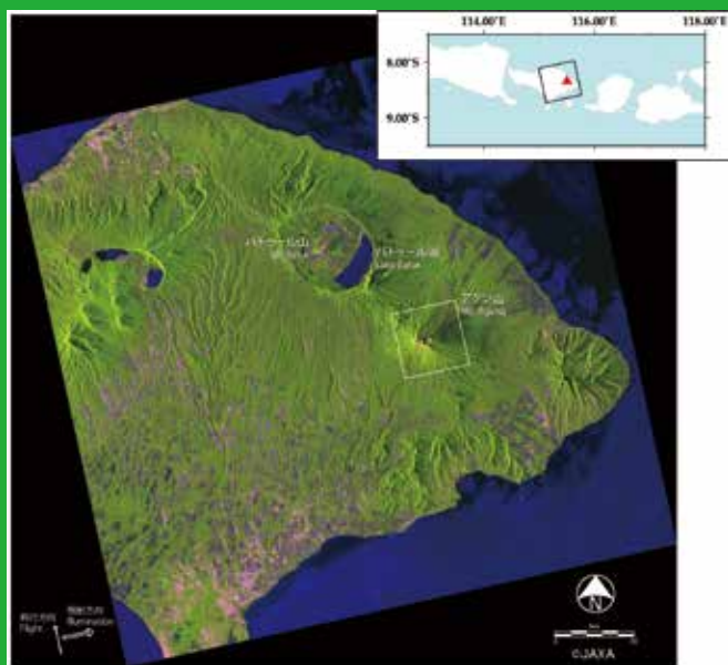
The figure above shows the PALSAR-2 observation area on 1 December 2017 (Red triangle on the top right of the figure: Location of Mount Agung; Black frame: Observation range). The color composition is as follows: HH polarization data observed through the ALOS-2 Stripmap 10m mode (dual polarization) in red, HV polarization in green, and HH polarization/HV polarization ratio in blue. The areas in blue and black show water and bare ground respectively, areas in green denote vegetation, and the localized areas in bright green and purple show town and urban areas.
